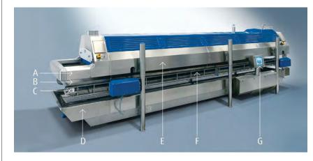
The CRYOLINE **CW IQF** tunnel freezer features (A) fully welded SS sloped surfaces, (B) continuous operation with surfaces that easily drain liquids, (C) a CIP-ready beltwashing option, (D) internal sloping sides, (E) a top that raises for cleaning and maintenance, (F) rolling-wave belt and (G) autologging of operating parameters. Source: Linde LLC.
